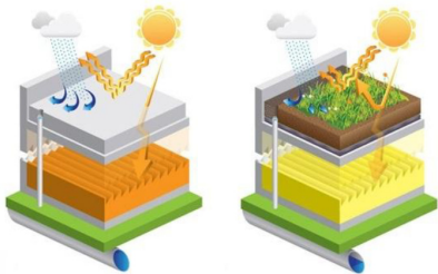
Figure 2: A traditional roof (left) and a green roof (right). Green roofs provide rainwater storage and heat absorption, resulting in reduced strain on conventional stormwater infrastructure and more insulation from incoming solar radiation. 51
